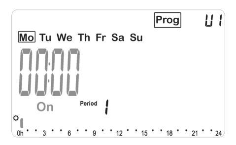
Adjust the hour of the first step of the program with (-) or (+).
