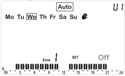
To manually override the schedule settings temporarily press (OK) and use (-) and (+) keys to toggle between 'off' and 'on' modes, press (OK) to confirm. If overriding the (Hand) symbol will be displayed. The set schedule will return at the next period change.
