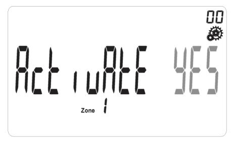
By displaying a flasing "Yes", this means that Zone 1 is active. By displaying a flashing "No", this means that Zone 1 isn't active. Select "Yes" or "No" with (-) and (+) keys.
