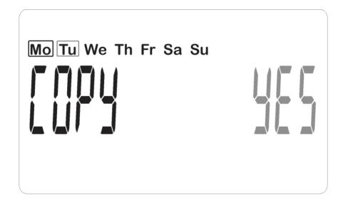
You can scroll between "Yes" and "No" using the (+) and (-) keys. Pressing the (OK) button will accept you selection. You can copy to each day individually or scroll to "No" and create new programmes as previously.
