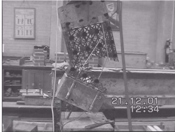
**Figure 2b, Tensile test at failure**
