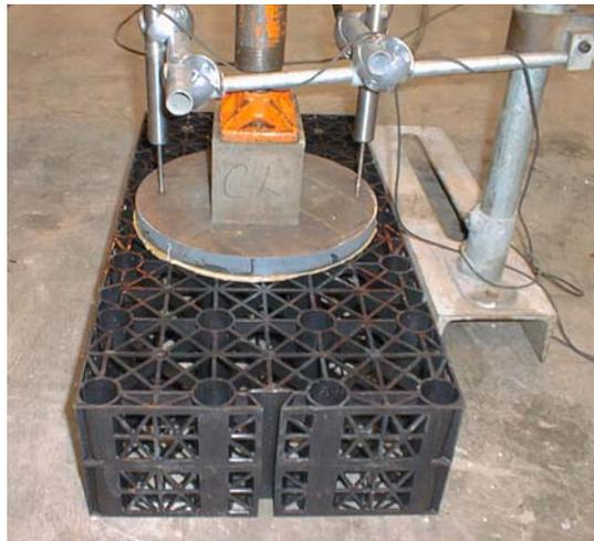
**Figure 2a, Compression testing**
