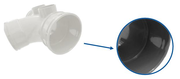
The downstream socket shows a shoulder stop at the base, this is to help a solvent weld bead to form, thereby maximising the solvent welds performance.
