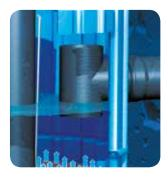
**4.** Situated above the filter element is an oil retention unit which removes the remaining contaminants from the surface water run-off. The clean water then flows via the outlet to the soakaway or watercourse.
