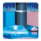
2. The hydrodynamic separator converts the radial flow to generate particle sedimentation to remove heavy debris and silt from the contaminated water. The sediment is then retained in a silt trap chamber below the separator for easy maintenance and access.
