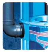
1. Contaminated surface water run-off is fed into the basal section of the filter. The angled inlet generates a radial flow pattern.
