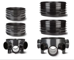
Ridgidrain Inspection Chambers are sold in component parts to be assembled on site. The base units are connected to Ridgidrain pipes using adaptors to form a watertight seal. Side risers are used to build the chamber to the necessary height and can easily be cut to the correct level using a fine tooth saw. A seal ring is used to ensure a leak tight joint. Cover and frames are available in a range of load classifications.
