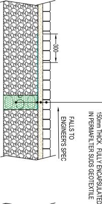
POLYPIPE PERMAFOAM CHECK GATE PROTECTION FLEECE ON BOTH SIDES
