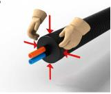
Press the shrink cap on the water and jacket pipe. Use protective gloves as the end cap is now hot.
