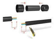
Remove carefully the jacket pipe and insulation layers to avoid damaging the medium pipe. The length of the naked medium pipe is marked with A. The length is depending on the diameter of the carrier pipe.
