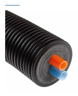
Highly flexible, pre-insulated piping system, combining both the flow and the return medium pipes in the same jacket pipe, primarily intended for the transport of heating water or other heat-transfer media in underground distribution networks.
