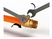
Tighten the large bolt until both clamping ring halves touch each other.
