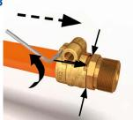
Slide the clamping ring over the fitting, until both jaws pass over the fitting collar.
