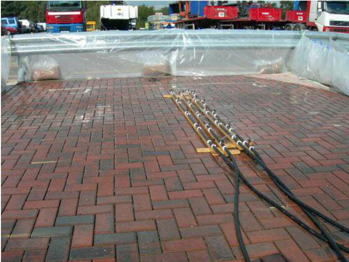
Figure 8.1: Simulated rainfall on block paving (Bay 1)
