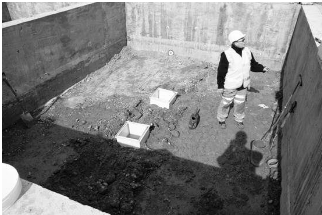
Figure 8.13 Infiltration tests in as-found soil.
