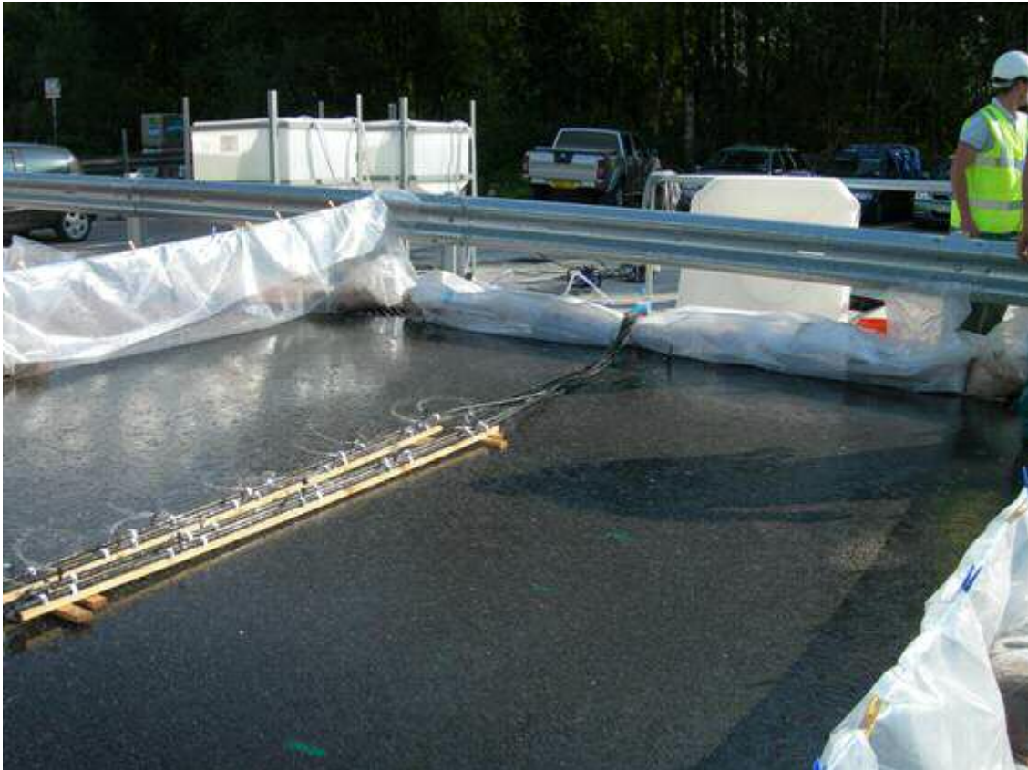
Figure 8.2: Simulated rainfall on asphalt (Bay 2)
