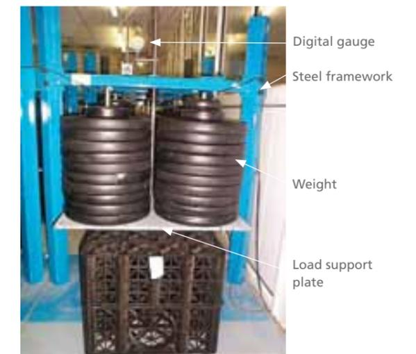
Figure 11 Creep test rig
