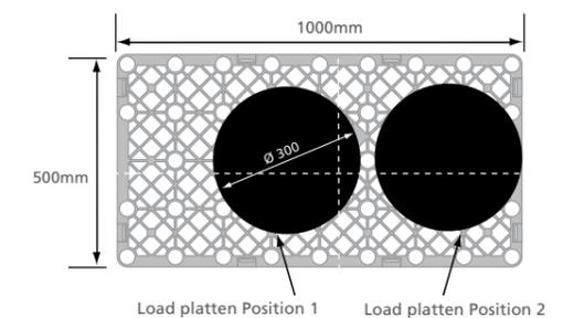
Figure 10 Position of load platens; point load resistance
