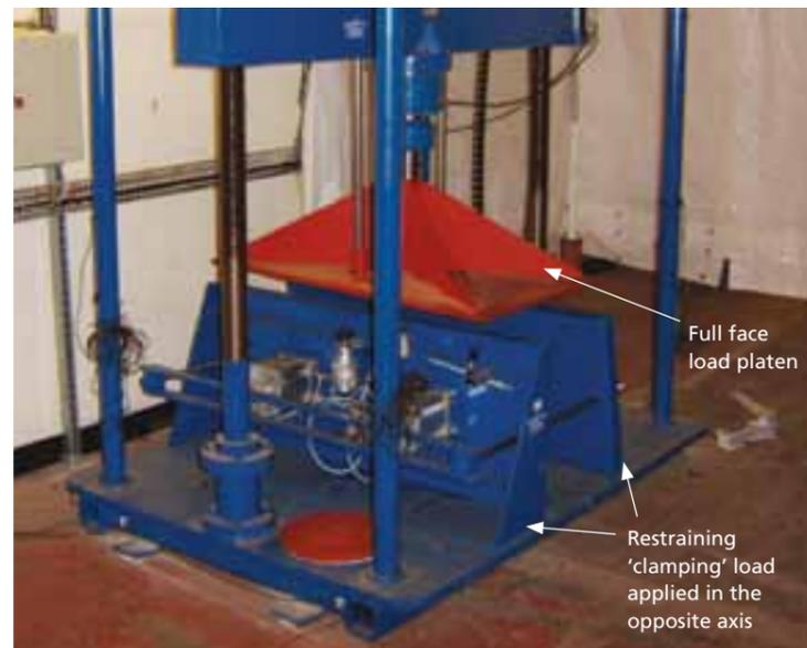
Figure 8 Compression test rig
