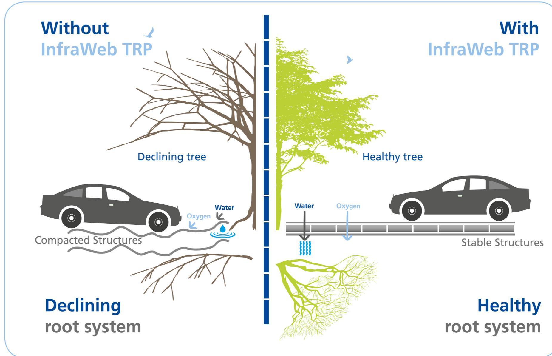
BS5837 (2012) recommends the use of a 3 dimensional cellular confinement system for use as appropriate subbases for new hard surfacing over the RPA of existing trees.
