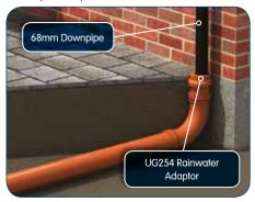
Square Downpipe discharging into drain via Square to Round Adaptor
