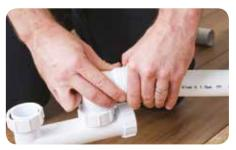
**6.** A final inspection of the connection is required to make sure the connection has been made by pulling on the pipe and fitting. This may not be suitable in certain applications.
