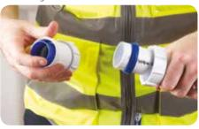
Polypipe's blue Fit-Rite™ insertion aid can be left in the body of the fitting if you are connecting to solvent weld and Push-fit pipe. If you are connecting to metal pipe or distorted plastic pipe you can remove the pipe insertion aid.
