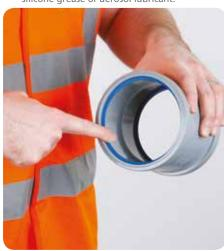
Insert the pipe or fitting into the socket and then withdraw it by approximately 10mm to allow for expansion of the pipework.
