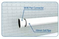
Pan connectors are manufactured from polypropylene and all versions have a 110mm spigot outlet for connection to a ring seal soil system socket. This type of connector is not suitable for solvent welding.
