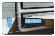
For buildings between 5 and 20 storeys, the ground floor appliances should connect direct to drain or to their own soil stack.
