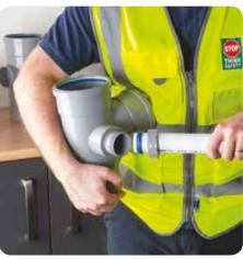
**4.** Tighten the compression nut by hand and then once tight make an additional ¼ turn.
