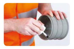
4. Apply a coat of Polypipe solvent cement to both surfaces to be jointed using the brush applicator provided in the lid. The cement should be applied along the length of the spigot and not around its diameter.
