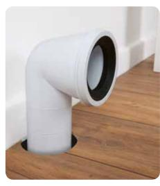
2. Place the finned section of the pan connector into the soil pipe or soil fitting that should be situated below the floor level. Depending on the installation it may be more suitable to install the pan connector on the toilet first.
