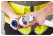
3. Place the threaded nut first onto the pipe, then the blue washer. Finally push the seal onto the pipe with the seal facing into the fitting.
