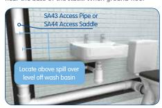
appliances are connected to the soil stack, the access point should be sited above the spillover level of the appliances.
