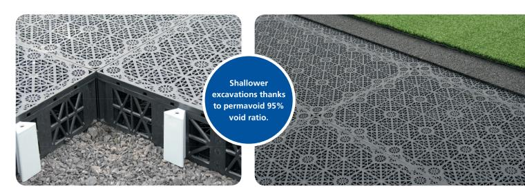
This design solution enables substantial quantities of water to be attenuated within the pitch construction, with no need to install expensive attenuation tanks elsewhere on-site. The Permavoid blanket has a 95% void ratio (much higher than a traditional stone sub-base design).
