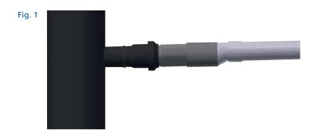
Adapting from one material to another can sometimes require a number of different fittings. An example shown (Fig. 1) shows a solution of bringing 32mm PVC waste into a 40mm Terrain FUZE HDPE branch. As you can see there is a requirement for a number of fittings to make this adaption.
