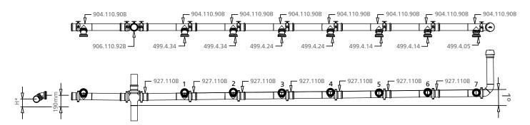
Float laid to a Fall of 1° (17mm drop/1 metre run)
