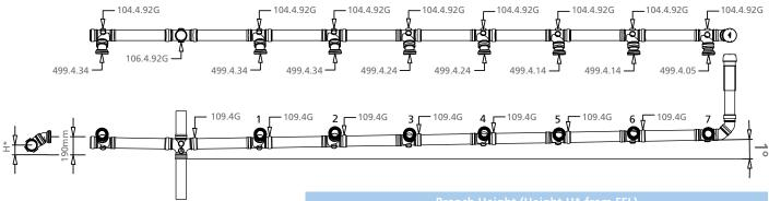
Float laid to a Fall of 1° (17mm drop/1 metre run)
