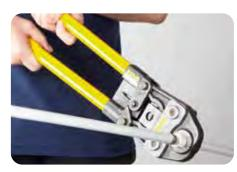
Extension pieces are included with the Eco Press if extra leverage is required to completely close the tool. Only when the tool has been completely closed with the two stops touching is the fitting fully secured. The levers can then be opened and the fitting will be released from the jaws.
