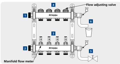
First, close the isolation valves (1&2) to the system. Then connect hose pipes to the manifold drain/ fill points.
