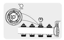
Balancing the system is simply done using the key provided, remove the blue caps and turn each circuit to the required / designed flow rate indicated in litres per hour. The Automatic flow control technology will then constantly adjust each circuit to the desired flow rate.
