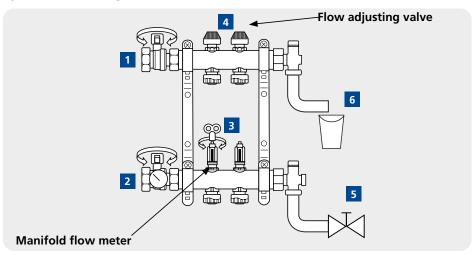
First, close the manifold isolating valves (1) and (2). Then connect a hose pipe to the manifold return drain off point (6) and take to a drain. Connect a second hose pipe to the manifold filling point (5) and attach to mains cold water supply (3 bar max). The connections to the manifold drain and fill points are ¾" BSP. Use flexible ¾" tap connectors for the simplest method of connection.
