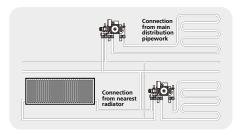
The diagram above shows the ZRU connected to operate with the boiler on/off firing. Due to the quick response of low mass systems (Overlay™, Overlay™ Lite, MHP, etc.) this is likely to be suitable. Using this method for solid floor installations may require the timings of the existing heating to be altered to allow the underfloor heating system to reach comfort temperature.
