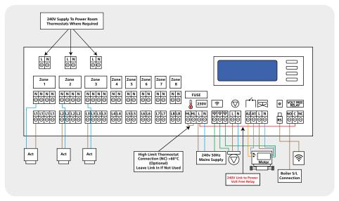
If fitting without a Zone Valve, ensure that the factory fitted link across terminals A1 and A2 is in place.
