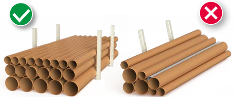
DIAGRAM 3: Correct and Incorrect way to store pipes
