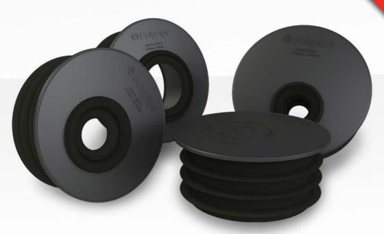
Polypipe In-floor Waste Adaptors are a quick and convenient method of adapting waste and overflow pipes to PVCu, Cast Iron and Clay drainage or soil pipes. The finned external gasket gives a water, air and odour tight seal to the internal bore of the drainage pipe.
