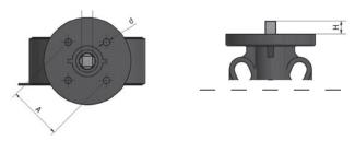
The regulating notch plate/handle can be easily removed for the mounting of an electric or pneumatic actuator, or for the fitting of a manual gearbox.
