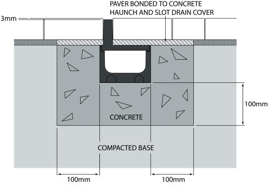
The trench size should be calculated according to the above diagram.
