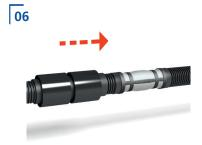
Slide over the straight covering jacket pipe, until both ends of the pre-insulated pipe are covered. Then slide over both shrinking sleeves, each of them covering half straight covering pipe and half jacket pipe.
