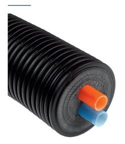
Highly flexible, pre-insulated piping system, combining both the flow and the return medium pipes in the same jacket pipe, primarily intended for the transport of heating water or other heat-transfer media in underground distribution networks and hot and cold water supply.
