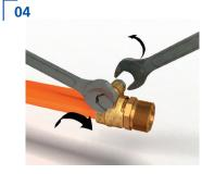
Tighten the bolt until both clamping ring halves do reach/ touch each other.
