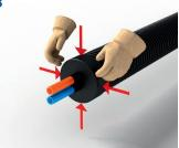
Press the shrink cap on the medium and jacket pipe. Use protective gloves
