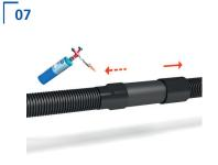
Heat up softly both shrink sleeves and press using protective gloves.
