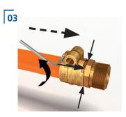
Slide open clamping ring to fitting, until both jaws passed the fitting collar. Unscrew the small bolt by using a hex key.
