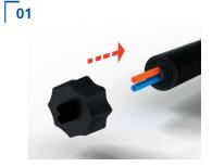
Dismantle the jacket pipe and slide the shrink cap on the jacket pipe.
