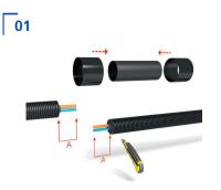
Remove carefully the jacket pipe and insulation layers to avoid damaging the medium pipe. The length of the naked medium pipe is marked with A. The length is depending on the diameter of the carrier pipe.
