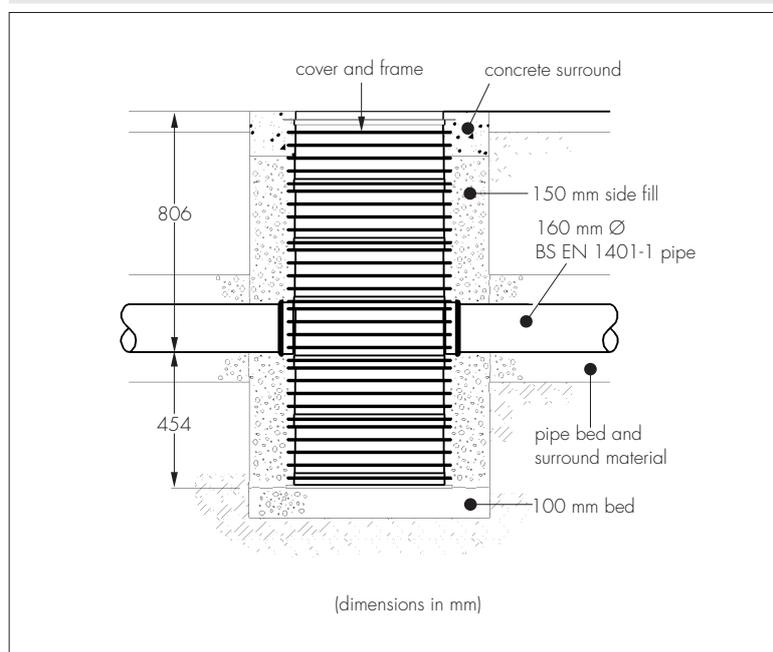
11.5 For all flow control devices it is sensible to incorporate access (via a manhole or similar) to the location of the pipe entry, orifice or vortex control. This will enable easy removal of any blockage. The orifice itself may be protected by a debris screen.
