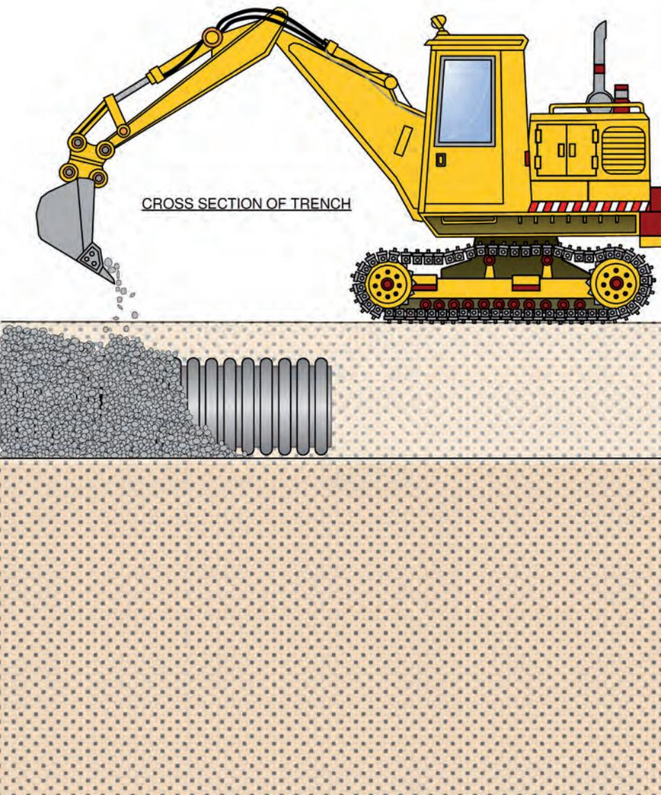
The diagram shows a yellow tracked excavator positioned on the right side of a trench. The excavator's arm is extended, and its bucket is dumping material into the trench. The trench contains a pipe with a joint. The pipe is surrounded by a layer of gravel, and the rest of the trench is filled with a sandy material. The excavator is labeled 'CROSS SECTION OF TRENCH'.
