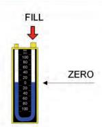
Allow pressure to stabilise for around 5 minutes increasing the pressure to 100mm/wg if it drops
