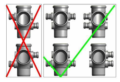
For fittings within the Terrain range which have 4 boss connections there are a number of permissible and impermissible configurations possible. The images on the left show configurations which are and are not allowed.
