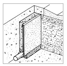
• THIS DETAIL SHEET RELATES TO LINFLEX 6 FIN DRAIN, A FIN DRAIN TYPE 6 AS DEFINED IN THE MANUAL OF CONTRACT DOCUMENTS FOR HIGHWAY WORKS (MCHW), VOLUME 3, DRAWING NOS F18 AND F19.
