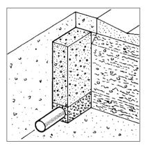
• THIS DETAIL SHEET RELATES TO LINFLEX 9 (FOR USE IN A TYPE 9 NARROW FILTER DRAIN) AS DEFINED IN THE MANUAL OF CONTRACT DOCUMENTS FOR HIGHWAY WORKS (MCHW), VOLUME 3, DRAWINGS NOS F18 AND F20.
