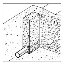
• THIS DETAIL SHEET RELATES TO LINFLEX 8 (FOR USE IN A TYPE 8 NARROW FILTER DRAIN) AS DEFINED IN THE MANUAL OF CONTRACT DOCUMENTS FOR HIGHWAY WORKS (MCHW), VOLUME 3, DRAWINGS NOS F18 AND F20.
