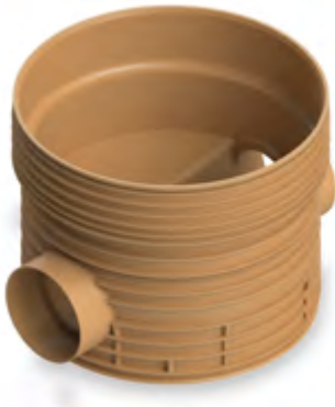
IC6BS6 600mm dia. base straight channel and single inlet for 110/150/160mm BS EN 1401 Underground pipes when used with appropriate adaptor
