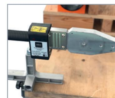
1. Check the hand welding tool and relevant male/female irons for damage.
