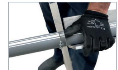
Support the pipe during cutting to prevent movement, allowing the end to be cut as square as possible.
