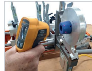
3. Turn the machine on and allow the hot plate to reach a temperature of 260°C. This should take between 10 and 30 minutes.
