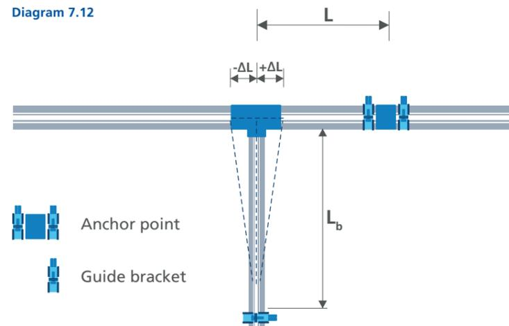
Compensating for changes in length using an expansion leg, 'L<sub>b</sub>'
