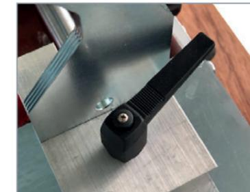
4. While waiting for the hot plate to reach the required temperature, adjust the pipe and fitting clamps to approximately the correct level, using the pipe and fittings as a guide.
