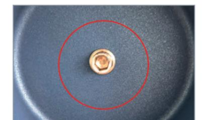
4. While the device is heating, re-tighten the bolts holding the male and female irons on to the hot plate.
