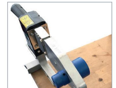
3. Plug the hand welding device in and allow it to reach the correct welding temperature. This should take between 10 and 30 minutes.
