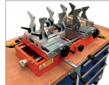
1. Place the socket welding machine on a secure bench. Set the correct diameter of the pipe being socket welded.
