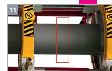
Under no circumstances must the ends of the pipe be touched or contaminated from this point forward. If they are then they must be re-planed.
