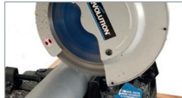
For a cut that requires minimal finishing work, use a 60-100T circular tungsten carbide blade suitable for cutting plastic.
