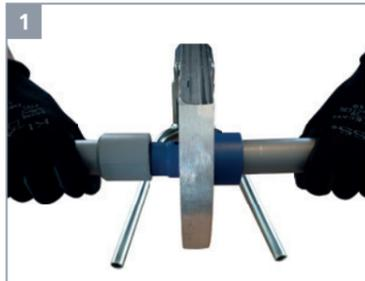
1. Pre-mark the insertion depth on each pipe. Push the pipe into the female iron and push the fitting on to the male iron. Insert to the mechanical stop. Do not twist the pipe or fitting.
