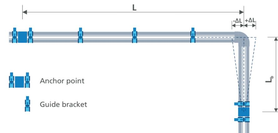
The equation to calculate distance 'L<sub>b</sub>' is given as:
