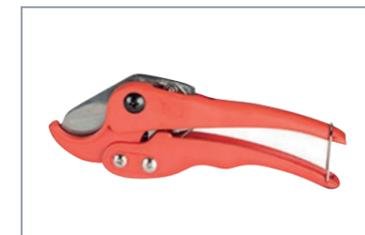
Ratchet cutters with a sharp, pointed blade should be used for smaller pipe sizes, this prevents the pipe from deforming during cutting.
