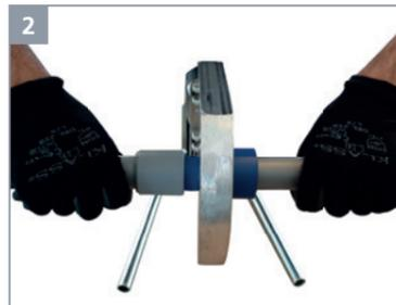
2. Once the pipe and fitting both reach the mechanical stop, apply heat for the required time.
