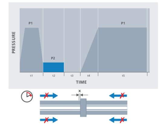
Diagram 6.13 – t3 Removing the heating element
