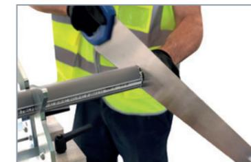
Hand saws may be used, however it is crucial to ensure the cut is square, and the edges are as smooth as possible.
