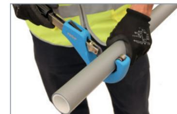
Alternatively, tube cutters can be used. Ensure the cutting wheel has a radius greater than the pipe wall.
