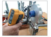
3. Turn the machine on and allow the hot plate to reach a temperature of 260°C. This should take between 10 and 30 minutes.
