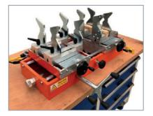
1. Place the socket welding machine on a secure bench. Set the correct diameter of the pipe being socket welded.
