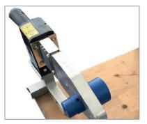
3. Plug the hand welding device in and allow it to reach the correct welding temperature. This should take between 10 and 30 minutes.
