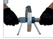
2. Once the pipe and fitting both reach the mechanical stop, apply heat for the required time.
