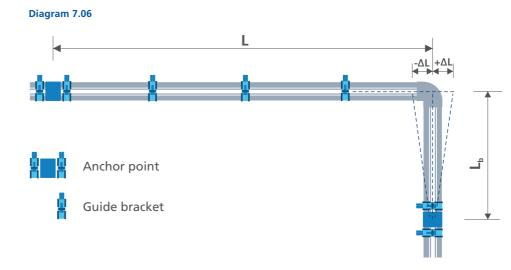
The equation to calculate distance 'L<sub>b</sub>'is given as:
