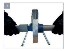
1. Pre-mark the insertion depth on each pipe. Push the pipe into the female iron and push the fitting on to the male iron. Insert to the mechanical stop. Do not twist the pipe or fitting.
