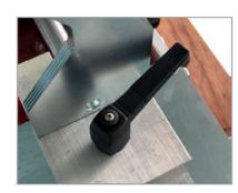
reach the required temperature, adjust the pipe and fitting clamps to approximately the correct level, using the pipe and fittings as a guide.
