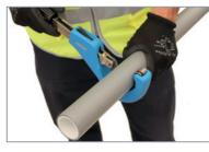
Alternatively, tube cutters can be used. Ensure the cutting wheel has a radius greater than the pipe wall.
