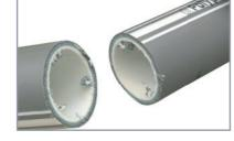
Once a cut is made, check the ends of the pipe for damage, both internally and externally. If any damage is identified, mark and remove the damaged area, cutting a few millimetres beyond the damage.
