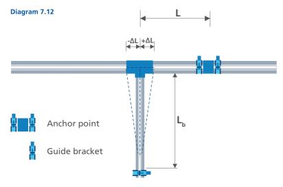
Compensating for changes in length using an expansion leg, 'L<sub>b</sub>'
