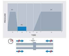
Diagram 6.13 – t3 Removing the heating element
