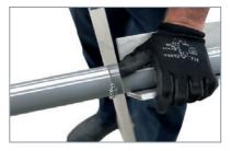
Support the pipe during cutting to prevent movement, allowing the end to be cut as square as possible.
