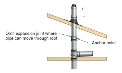
a) Above the highest branch connection to a foul and/or waste stack is free to move through a weather proof roof sleeve.
