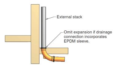
**b)** At the base of an external drainage stack that is connected to a drainage connection that allows movement through an EPDM sleeve.
