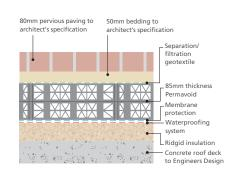
As the image above shows, the system can be installed in both warm and cold roof build ups and because the system forms a structural raft, the build up above the units can be as little as 50mm for un-trafficked paved areas. In addition, as the connected Permavoid Cells form a structural raft, the Permalock system allows for roof furniture - railings and plant, such as photovoltaic cells, to be fixed to the structural Permavoid raft without detriment to the roof waterproof membrane.
