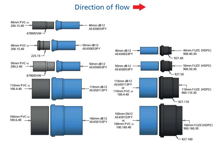
Note: Pipes to be chamfered and lubricated when being used with ring seal, use 9136.250L Silicone grease.
