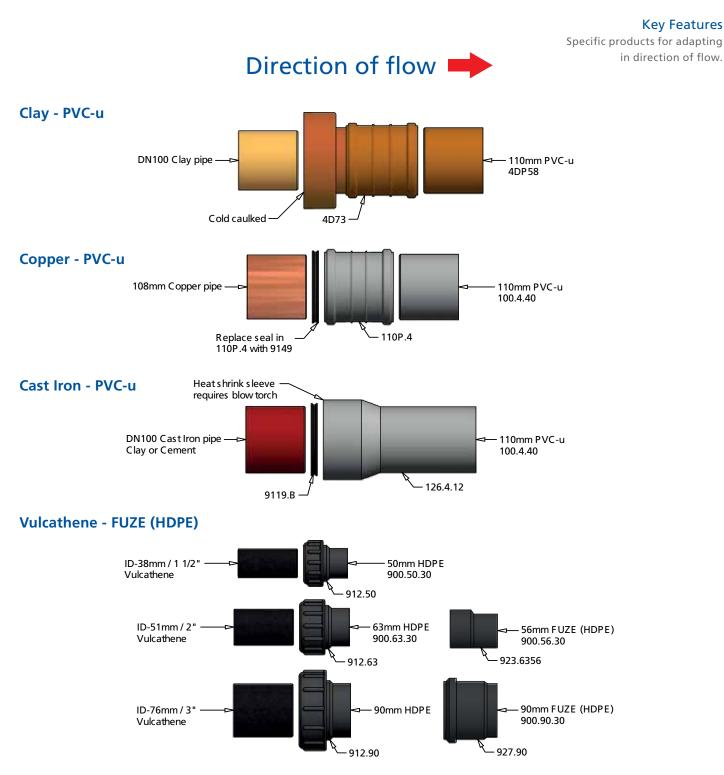
Note: Pipes to be chamfered and lubricated when being used with ring seal, use 9136.250L Silicone grease.
