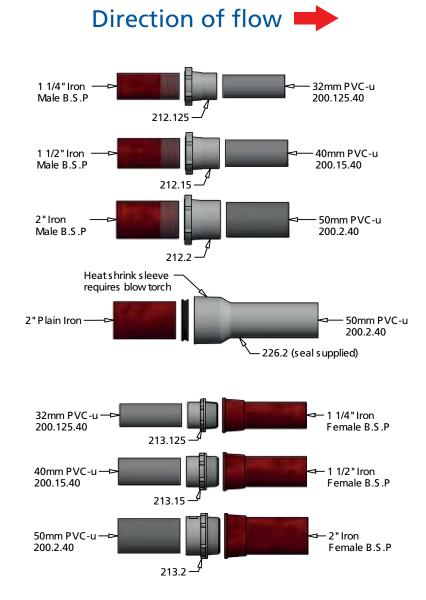
Note: Pipes to be chamfered and lubricated when being used with ring seal, use 9136.250L Silicone grease. References: 1. Terrain Soil and Waste Product Installation Guide. 2. BSEN12056 Gravity drainage systems inside buildings. Sanitary pipework, layout and calculation. For more information please call our **Technical Team on 01622 795200**.
