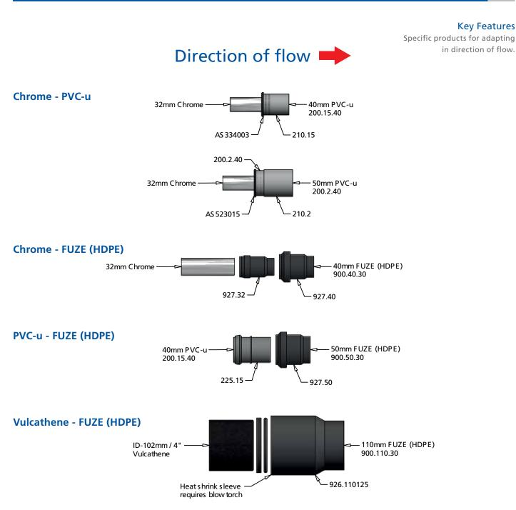
Note: Pipes to be chamfered and lubricated when being used with ring seal, use 9136.250L Silicone grease. References: 1. Terrain Soil and Waste Product Installation Guide. 2. BSEN12056 Gravity drainage systems inside buildings. Sanitary pipework, layout and calculation. For more information please call our **Technical Team on 01622 795200**.
