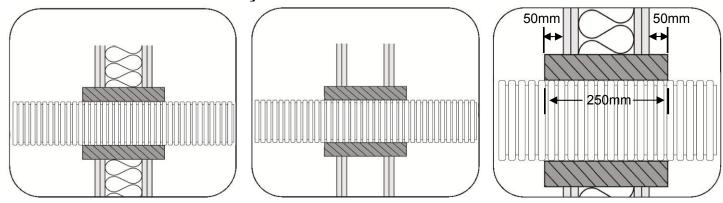
For timber stud partitions, seal must be ≥100mm from studs with ≥100mm of insulation (A1 or A2 to EN13501-1) between seal & stud
