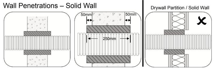
Rigid walls must comprise concrete, aerated concrete or masonry ≥650kg/m³ (Wall Type A) or concrete, masonry ≥1100kg/m³ (Wall Type B)
